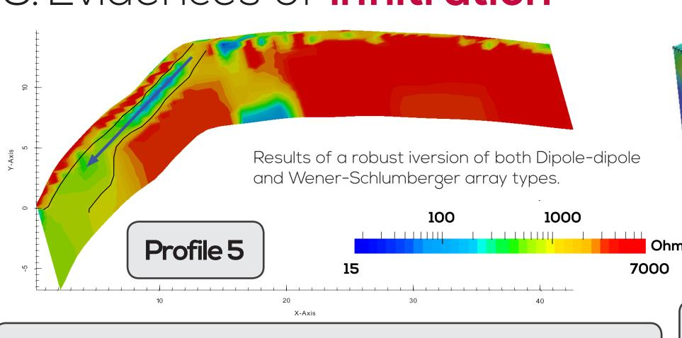
Profile 5 is located at the entrance of the cave along a side of the dolline. Electrodes were set following a stratigraphic unit. It is one of the most interesting site as it shows a low resistivity layer that appears to be related to water infiltrations through bedding joints.
